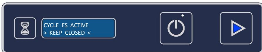
At the end of the cycle the luminous triangle turns green and another wash cycle can be started again. To select a different cycle time, press the "time selection button" (21) before the cycle is started; up to 4 programmable cycle times can be selected.
