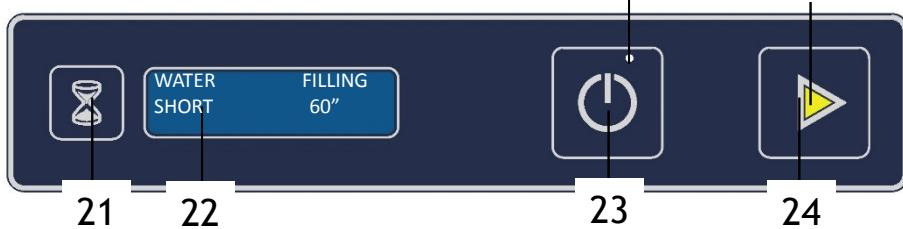
At the end of filling, heating starts and the display shows the tank and boiler temperatures.
