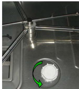
Make sure the salt does not spill and do not exceed the prescribed amount. After adding the salt, clean the seal, close the cap properly, eliminate any salt residues, remove the overflow and rinse the tank.
