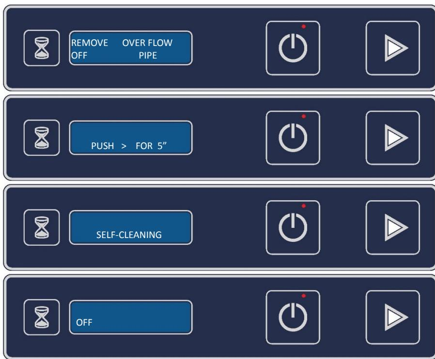
It is possible to set compulsory tank and boiler draining with intervals of 1 to 50 cycles. When the alert "FORCED DRAIN" appears, the dishwasher stops and remains in this state until complete draining of the tank.
