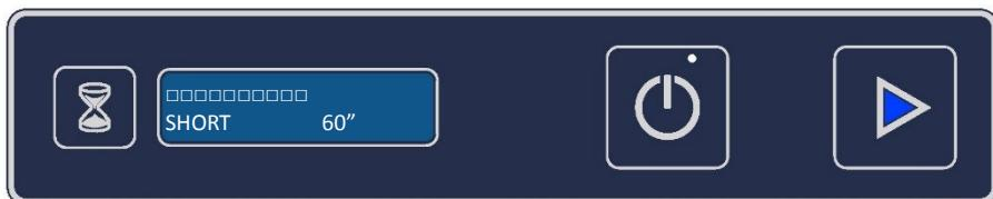
At the end of the cycle the luminous triangle turns green and another wash cycle can be started again. In versions with heat recovery unit, the washing chamber steam suction cycle starts at the end of the wash cycle.
