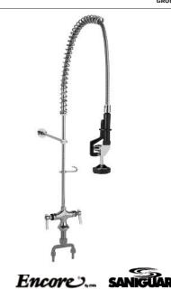
ENGINEERING SPECIFICATION: Polished Chrome Plated Brass Single Hole Deck Mount Pantry Faucet 1/4 Turn Compression Valves w/ Check Valves Lever Handles w/ SANIGUARD® Treatment S/S Flex Hose w/ Santoprene Reinforced Hose Stainless Steel Strain Relief – Patented O-Ring Seals - Patented Standard Full Spray Pattern 1.2 GPM Spray Face Included Hold open ring and hose hook included
